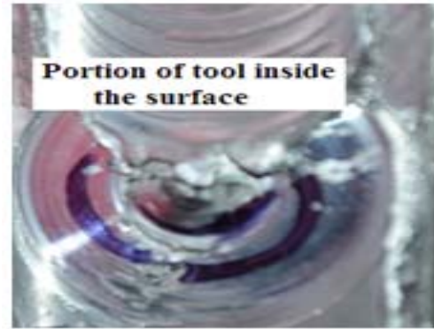
Fig. 2: Represents the breakage portion of tool embedded inside the surface of base.
