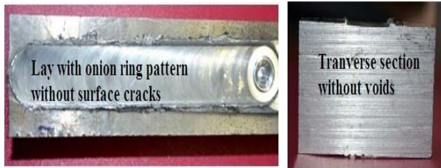
Fig. 4: Defect free SMMC (surface metal matrix composite) fabricated using FSP.
